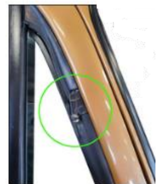
2 Piece vent window seals has exposed hinge pivot
