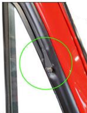
1 Piece vent window seals has covered hinge pivot
